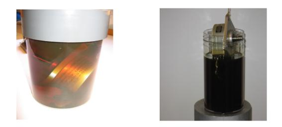
After 8 days the encoder was removed from the oil. After cleaning the exterior, the encoder was tested to determine if there had been any damage due to immersion.
