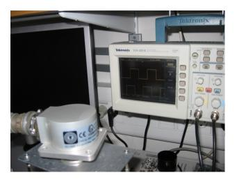
Test results indicated that the 2QEX encoder was working perfectly and that no damage or fluid ingression had occurred during immersion in oil.
